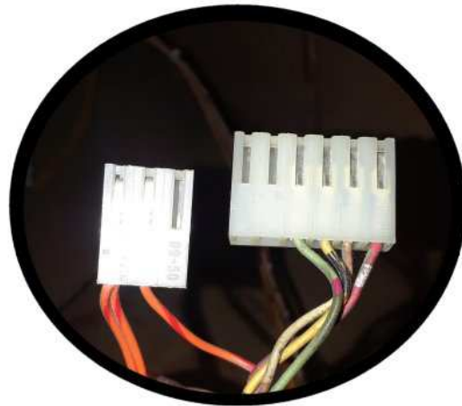
Photo: 3 and 6 pin video signal connectors disconnected.
