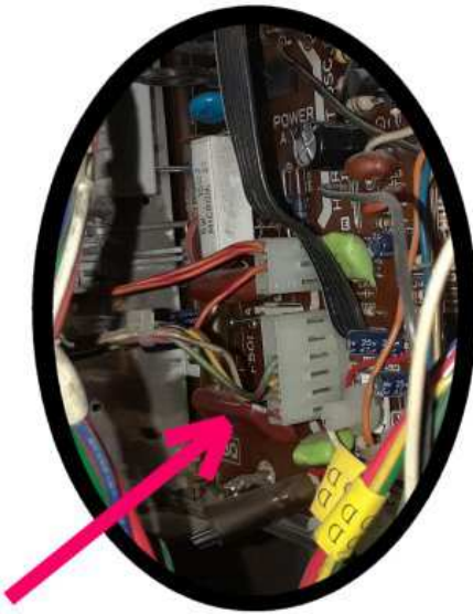
Locate and disconnect the video signal connectors.
