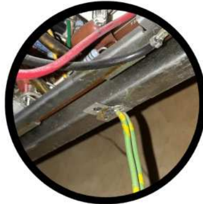
Locate and disconnect the green and yellow wire ground strap (if attached to the monitor frame)
